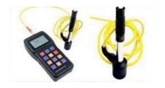
Press the Scale hardness key to switch HI, HB, HRB, HRC, HRA,HV, HS
